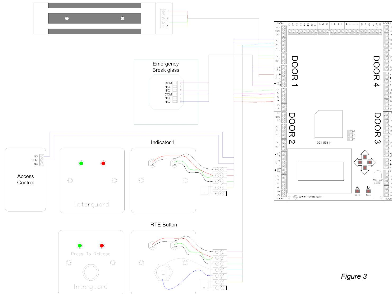
5.2 Wiring detail, locked doors with monitored locks, Access Control and RTE
